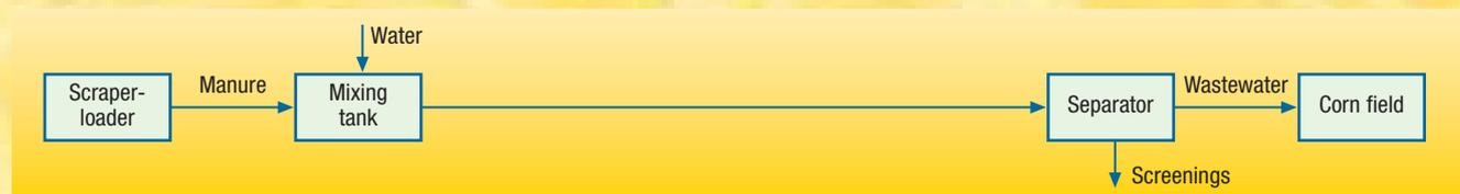
Figure 2. Schematic diagram of the Reference dairy-waste management system
