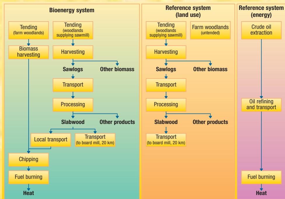
Figure 4. Main process steps involved in bioenergy and reference systems for wood fuel example.
