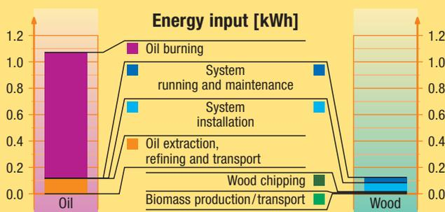
Figure 5. System 2: energy required to produce 1 kWh of useful heat.
