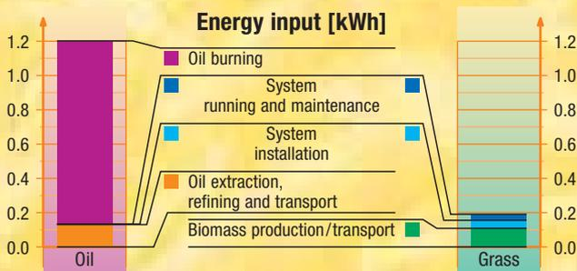
Figure 2. System 1: energy required to produce 1 kWh of useful heat.
