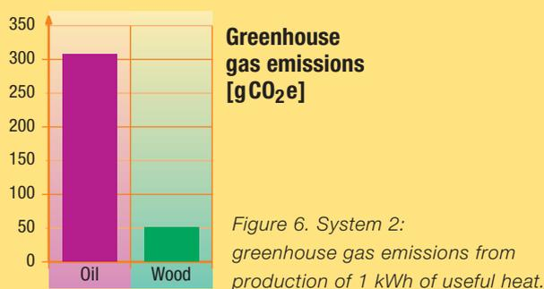
Figure 6. System 2: greenhouse gas emissions from production of 1 kWh of useful heat.
