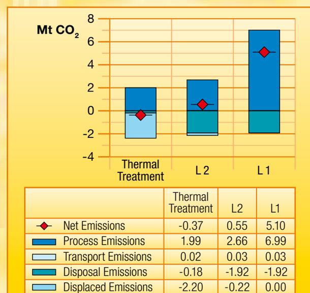
Figure 4: Total lifecycle greenhouse gas flux (Mt CO<sub>2</sub>) of each waste treatment scenario. Thermal treatment balance does not take into consideration the utilisation of process heat.
