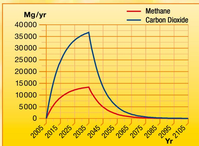
Figure 3: Annual CH<sub>4</sub> and CO<sub>2</sub> emissions from the landfill over 100 years
