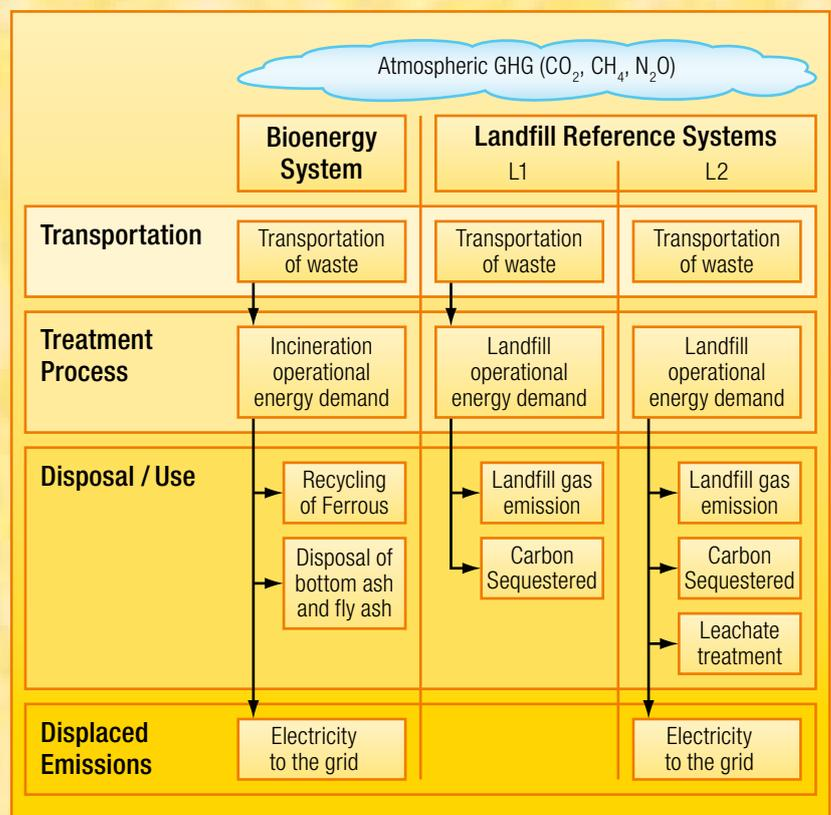
Figure 1: Lifecycle system boundary of the bioenergy system and the two landfill reference systems. The carbon sequestered in landfill contains both fossil (plastics) and biogenic carbon (wood, boards, paper etc).
