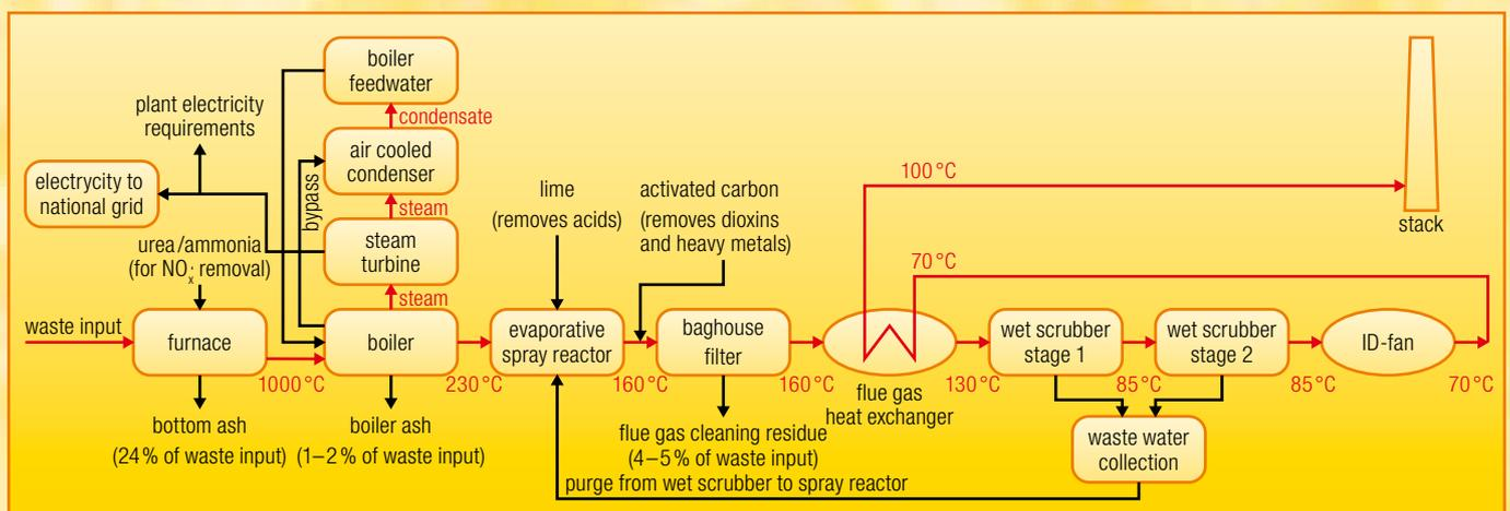
Figure 2: Process diagram of the proposed waste thermal treatment plant
